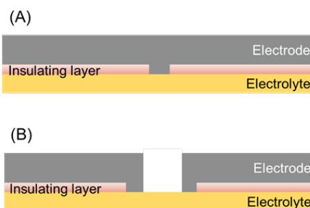
Figure 1. Schematic illustration of patterned thin film model electrodes used in this work. (A) Model electrode without triple phase boundary (TPB) and (B) model electrode with (TPB).
