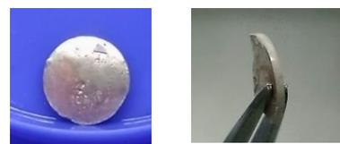
Figure 1. Digital camera images of a Li electrode on a garnet-type solid electrolyte pellet.
